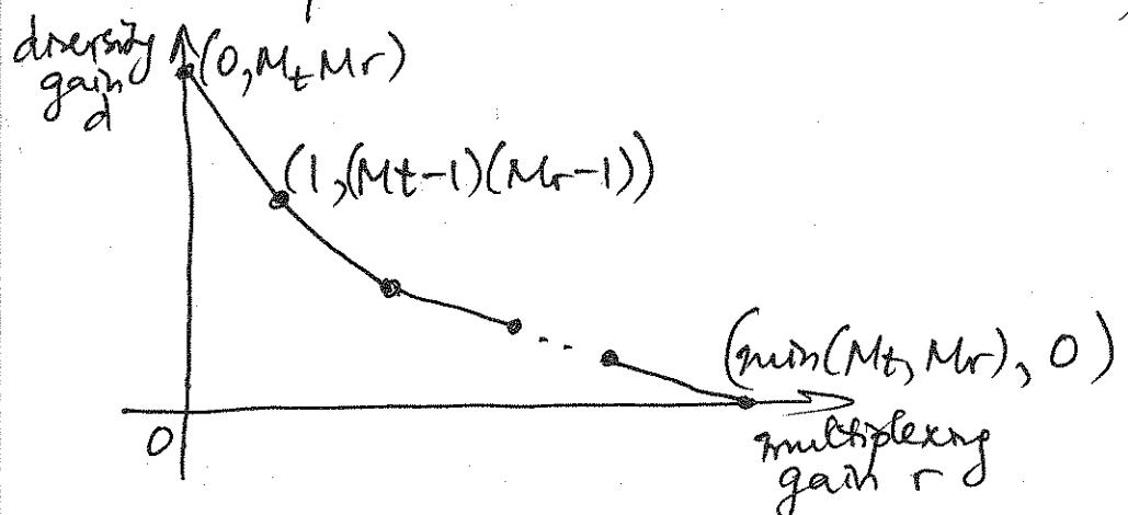
It is possible to adapt the diversity and multiplexing gain according to channel state. If the channel is bad, more antennas can be used for diversity, if the channel is good, more antennas can be used for multiplexing.
