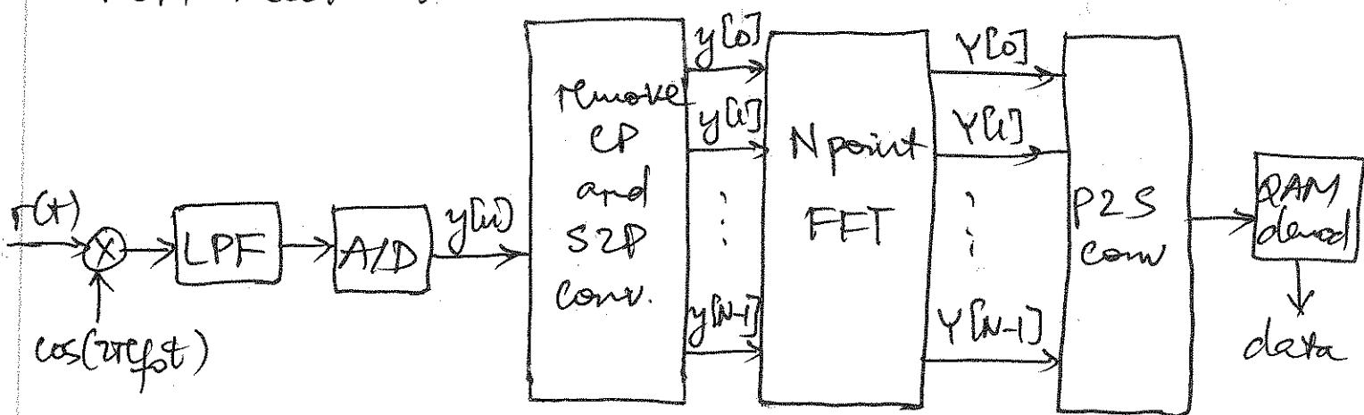
Instead of spending power to send the CP, one can also send zero-symbol CP, hence consuming no transmit power on the CP, and just add the tail of each receive sequence back to the beginning to create the circular convolution effect.
