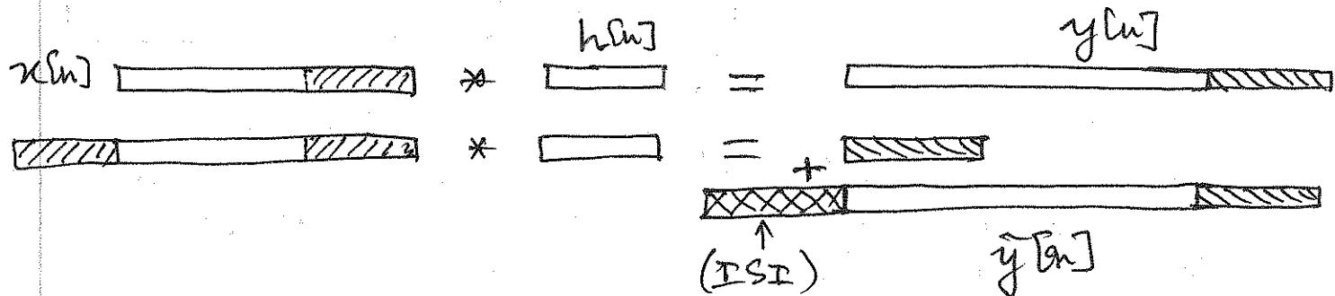
The cyclic prefix allows for the implementation of OFDM and DFT (FFT) operations but also adds overheads to the transmission.
