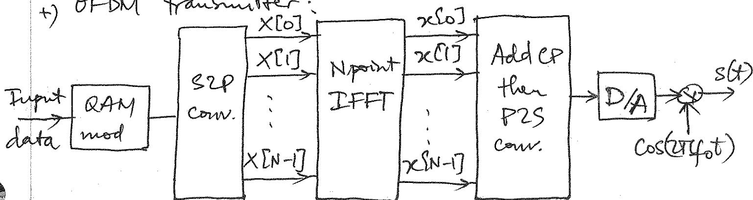
$X[k]$ : block of size  $N$  input (QAM) symbols is referred to as an OFDM symbol.
