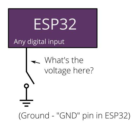
An input pin just reads whether the voltage (level) is above a threshold.
