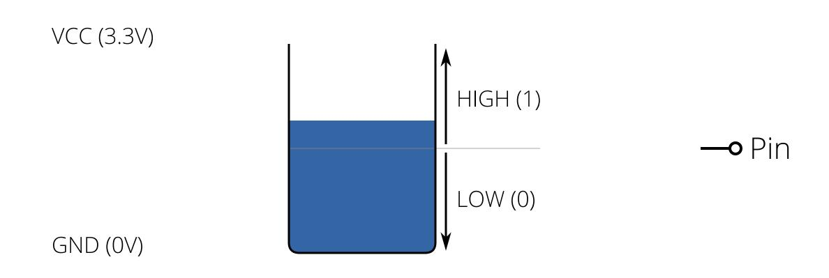
By reading the level, we can tell if the switch is making a connection to ground
