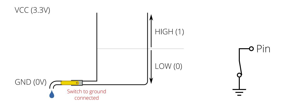
Except that when the switch is disconnected, we have no control over the level! We're at the mercy of the environment.
