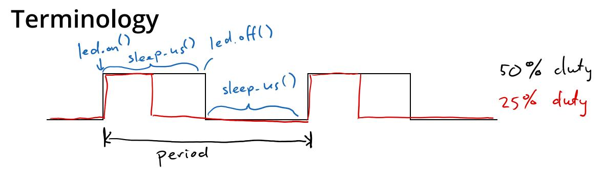
Pulse-width modulation (**PWM**): controlling something by varying the duty cycle (i.e, the width of the pulses)
