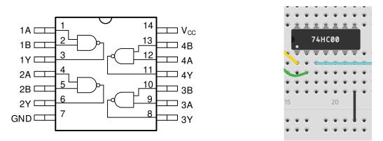
L7: Build the circuit below. You can use any of the four NAND gates in the package. Don't forget to wire up 5V (Vcc) and ground for the NAND chip! We've left those wires off the diagram, but the gate won't function without power!
