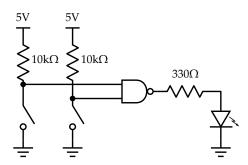
L8: Test your circuit to confirm that it works. Make sure you test all possible combinations of the inputs! Remember that pressing the button is a **low** input.
