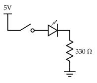
L4: What happens if you turn the LED around? (i.e., put the long lead on the ground side?)
