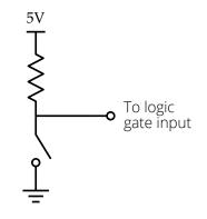
L6: Build the circuit above, and use the voltmeter at the point labeled "logic gate input" to confirm that the output switches between high (5V) and low (0V) when the switch is pressed.
