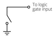
But when the switch is open (not pressed), then the gate is left "floating": neither high nor low, just disconnected. That may seem harmless, but it's not a valid input, and the circuit may behave unpredictably.
