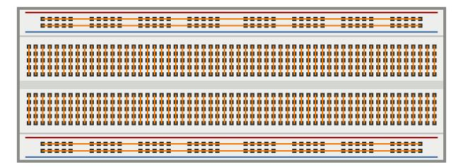
Each side of the breadboard also has two "rails" which run the full length of the breadboard.<sup>1</sup> By convention, we use the blue rails for the negative power supply (aka "ground") and the red rails for the positive power supply (aka "power", "5 V", or " $V_{cc}$ ").
