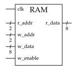
In this example, the 2 address bits specify four possible addresses, each of which refers to an 8-bit word, for a total of 32 bits of storage. Both the address width and the data width can be customized.
