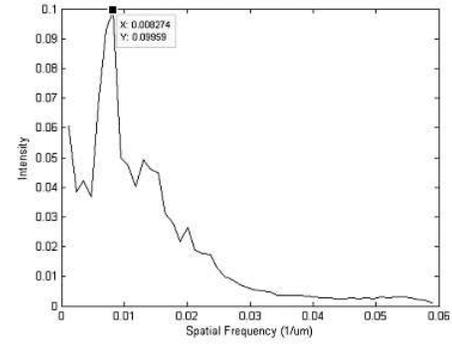
Fig. 5. Spatial frequency determined by two-dimensional fast Fourier transform of the image(Fig. 3) and integrating the FFT in the  $K_\phi$  direction.
