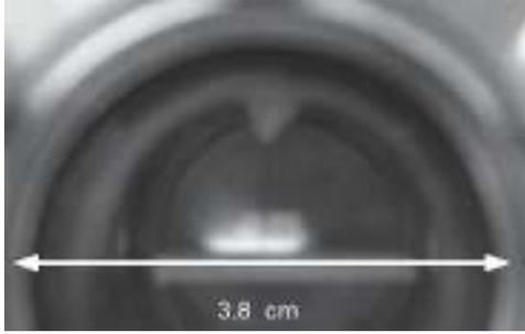
Fig. 4. Photograph of a 2 Torr argon microplasma viewed through the 3.8 cm side window
