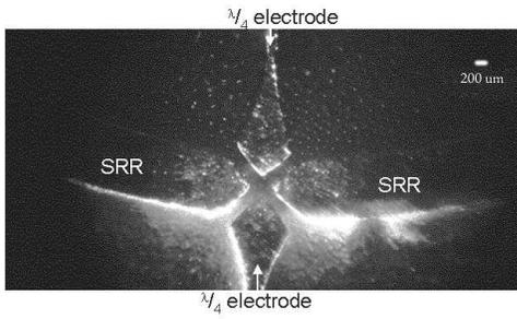
Fig. 3. Photograph of particles suspending in a 2 Torr argon microplasma
