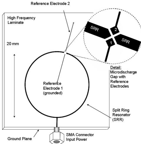
Fig. 2. Split Ring Resonator(SRR) and Reference Electrodes
