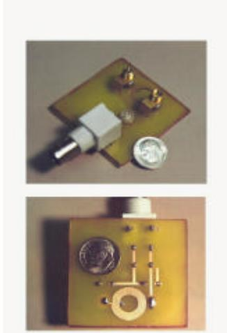
Fig. 2 - Top and bottom view of a miniature ICP circuit fabricated on a copper clad epoxy board. A U. S. dime is shown as a scale reference.
