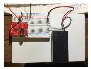
There's not really much to it. The big white mounting mounting board has the 3V battery pack and the breadboard mounted on it. The breadboard has our AD8232 board mounted on
