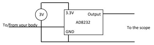
Your body's signals are quite low voltage and low power; the AD8232 board is largely a preamplifier that makes your body's signals strong enough to be easily displayed. The AD8232 needs battery power that is maximum 3.3V; a 3V battery works fine.
