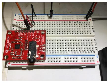
In the upper right, you can see the red and black wires (coming from the battery pack) driving 3V power and 0V ground into the breadboard.
