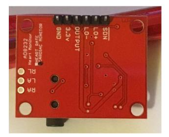
The AD8232 board has 6 pins sticking out from the bottom of the board, which go into breadboard row f, columns 3-8. Here's the breadboard with the AD8232 inserted and fully wired:
