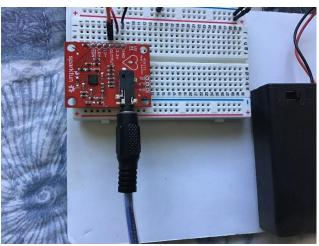
Note how tightly the plug fits into the socket. When you plug it in, be sure to support the AD8232 board with your fingers – the AD8232 board is attached to the breadboard with a few little pins that can easily break or bend if they're bearing any substantial force. If you don't push the plug in all the way, it might look like this:
