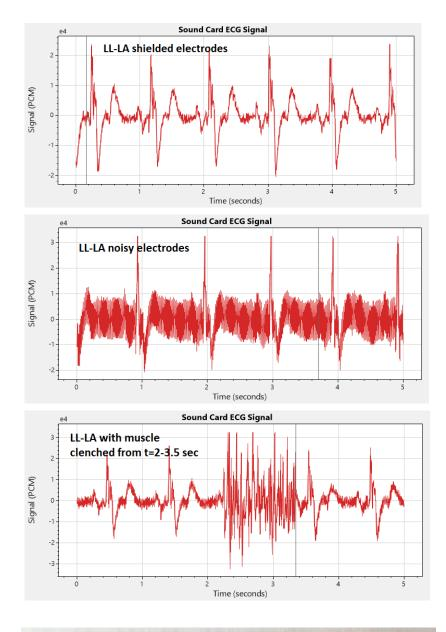
Lead III; left leg=+. Left arm = -. Nice shielded electrodes
