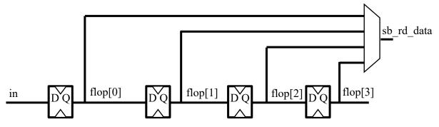
The slides don't give any detail on how to drive the select line(s) of the mux that drives the FIFO output data. The idea is to keep a count  $n_{items}$  of how many items are in the FIFO at any time.  $N_{items}$  would increment whenever you write the reference-model FIFO and decrement on reads. Since items are always written into flop[0], and move to the right as more items are added, the oldest item will always be in  $flop[n_{items}-1]$ .
